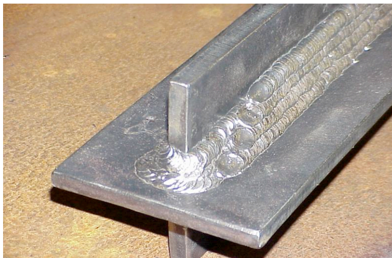
Example of a High Quality Weld
